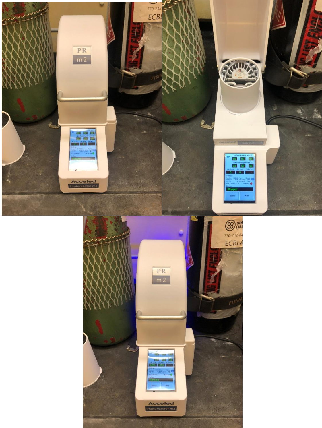
Figure 2. New photoreactor with integrated fan, LED light, and stirring functionalities. Top left: photoreactor in resting state (can be turned on and off with a switch on the side). Top right: inside of photoreactor contains reflective material and a cover to ensure reflection of blue light and minimization of blue light pollution. Bottom: photoreactor in use; shows minimal blue light exposure for reaction setup.
