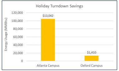
temperature days which reduce the potential savings since buildings had to be heated to maintain minium design temperatures. Emory's Atlanta and Oxford campus both saw a **3%** reduction from adjusting setpoints down. The holiday turndown managed to save **\$14,000** in utility costs over a 3 week period.
