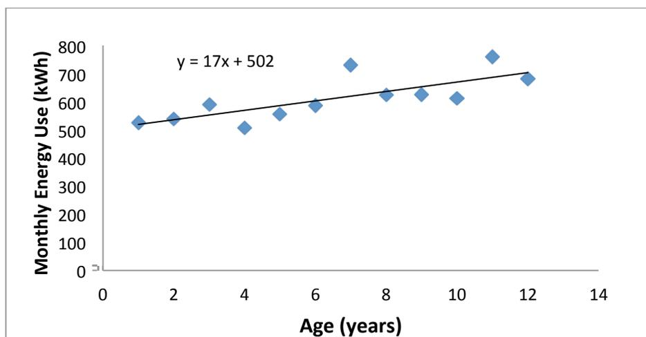
Figure 1 Energy consumption versus age for maintained 17.3 cubic foot (ft<sup>3</sup>) ULT freezers at a set point of -80°C (Gumapas and Simons, 2013)
