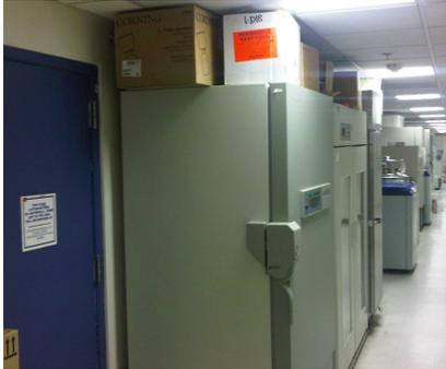
Each ULT freezer occupies 20-30 ft<sup>2</sup> of valuable space. Due to space constraints in labs, numerous ULT freezers are stored in hallways (figure 14). Most hallways are not designed not effectively remove heat generated from ULT freezers; therefore, ambient temperatures can be as high as 90°F (32°C). Operating ULT freezers at these ambient temperatures increases energy consumption by as much as 24% and increases the risk for a ULT freezer to fail, which puts samples at risk.
