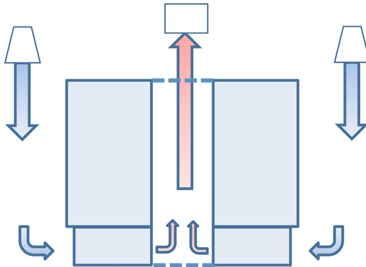
Figure 16 Reject heat management with panels and stratification.
